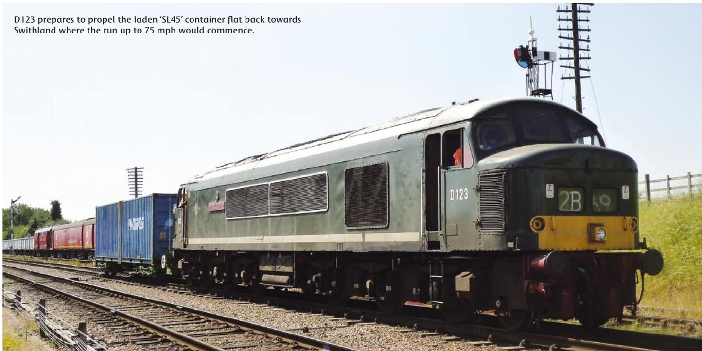
As part of the approval process for a new wagon, it is sometimes necessary to carry out a brake performance test. The level of testing required depends on what other tests have been carried out previously with wagons that have similar brake components and performance characteristics. In the past, these tests have been conducted on the 'mainline' railway, in recent years this has included the Down slow line between Crewe and Winsford. While this site is more than satisfactory, a
