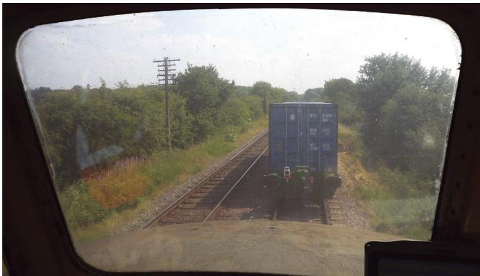
On the straight section of Down line towards Quorn station. The view from the rear cab of D123 shows the wagon having been slipped and slowing down to stop. During the tests there is a complete possession of the line in the test area.
